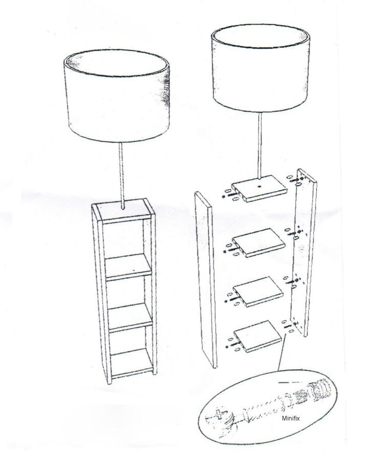
\*Fix the dowels and the minifx as it is shown in the picture. Use crosspoint screwdriver for the minifix
